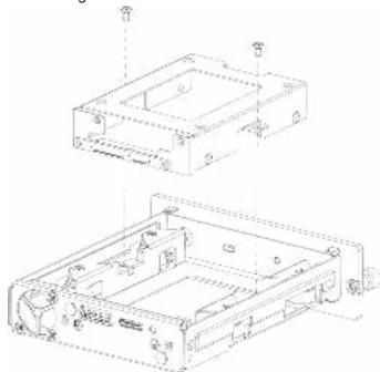
Step 6 Use four screws to fix the HDD and HDD holder, and install the HDD holder back to the Device.
