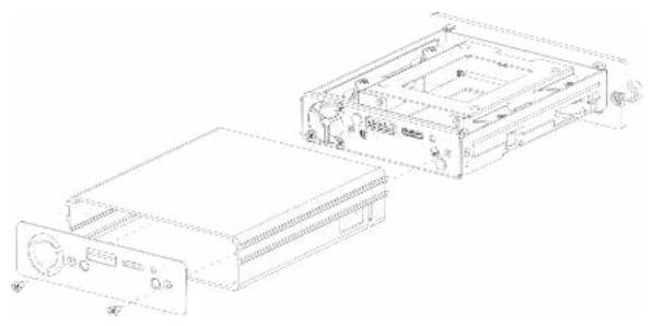
Step 5 Loosen two screws of the HDD holder and remove the holder.
