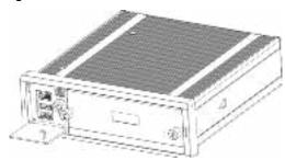
Step 3 Loosen the two screws at the front panel and take out the HDD carrier along the guide
