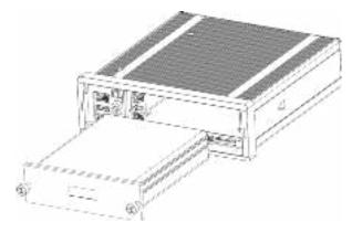
Step 4 Loosen two screws on the back panel of the HDD carrier, take out the rear carrier panel, and remove the HDD carrier enclosure.
