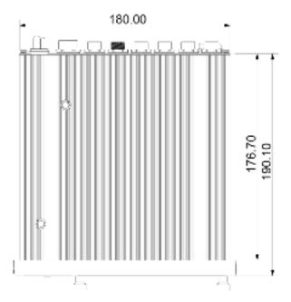
Figure 2-10 Hangers Installation Dimension Diagram (mm)
