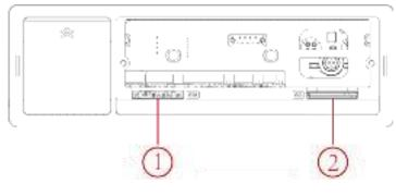
In Figure 2-16, ① is the SIM card slot and ② is the SD card slot.
