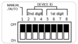
• Number notation of switch('2nd digits' can set with 3 switches and up to 7.)
