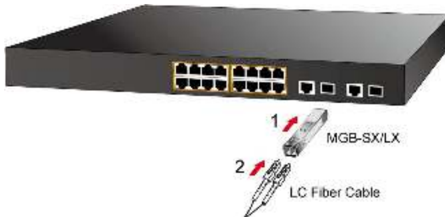
Figure 2-10 Plug in the SFP transceiver
