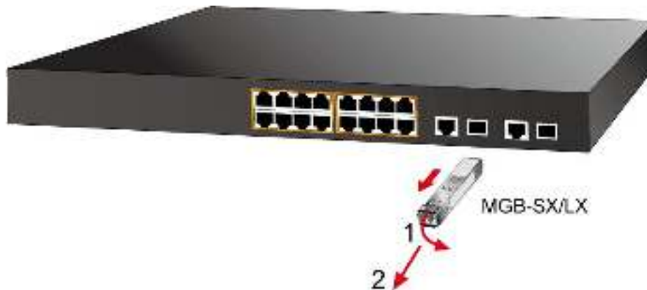
Figure 2-11 How to Pull Out the SFP Transceiver
