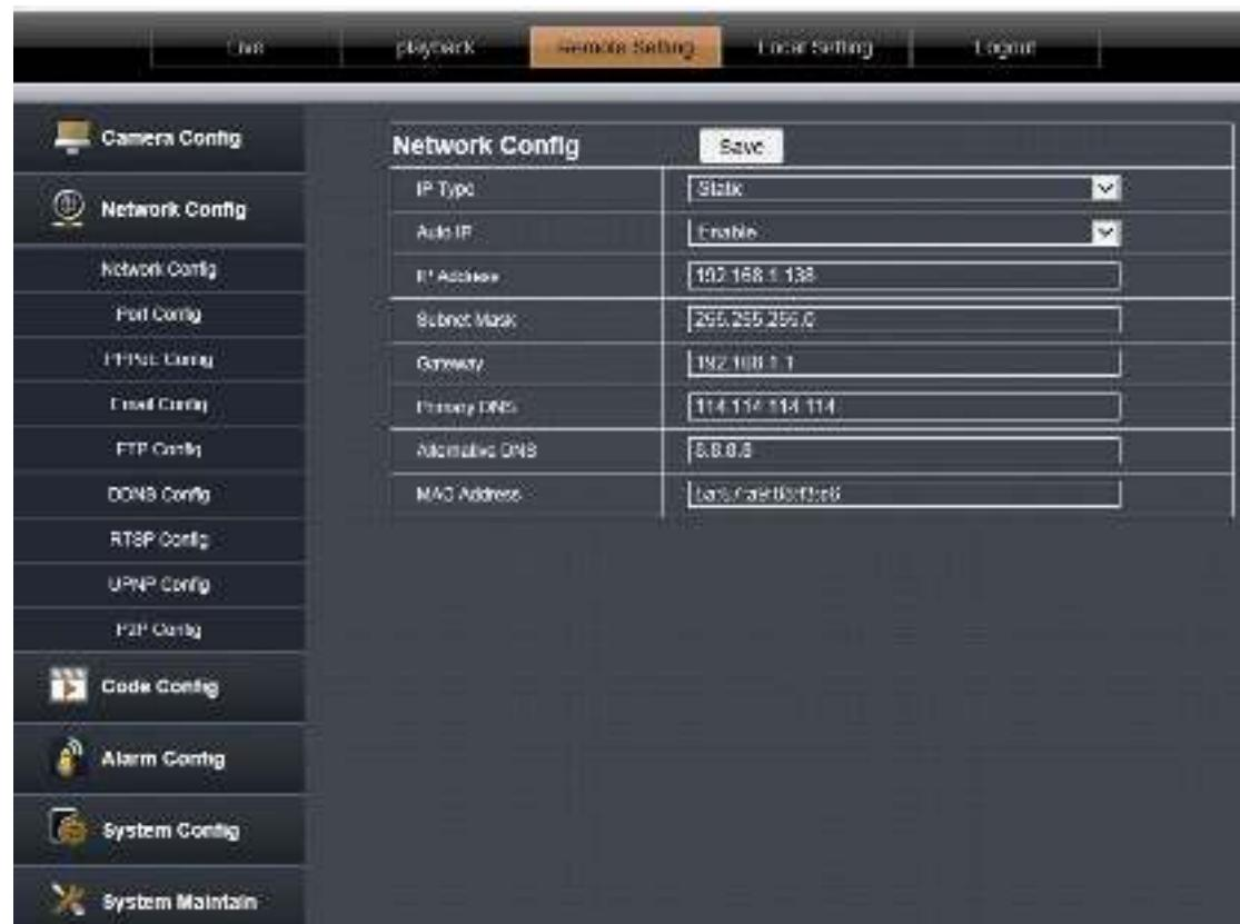
The screenshot shows the Amatek camera configuration interface with the 'Network Setting' tab selected. On the left, there is a sidebar with icons and labels for Camera Config, Network Config, Port Config, PPPoE Config, Email Config, FTP Config, DNS Config, RTSP Config, UPnP Config, P2P Config, Code Config, Alarm Config, System Config, and System Maintain. The main panel displays the 'Network Config' settings:
