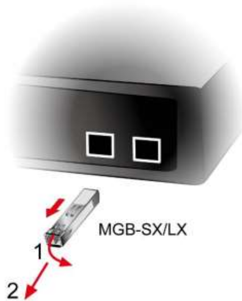
Figure 2-2-2 How to Pull Out the SFP Transceiver
