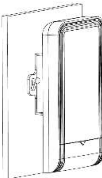
Figure 2-5 Wall Mounting Finished
