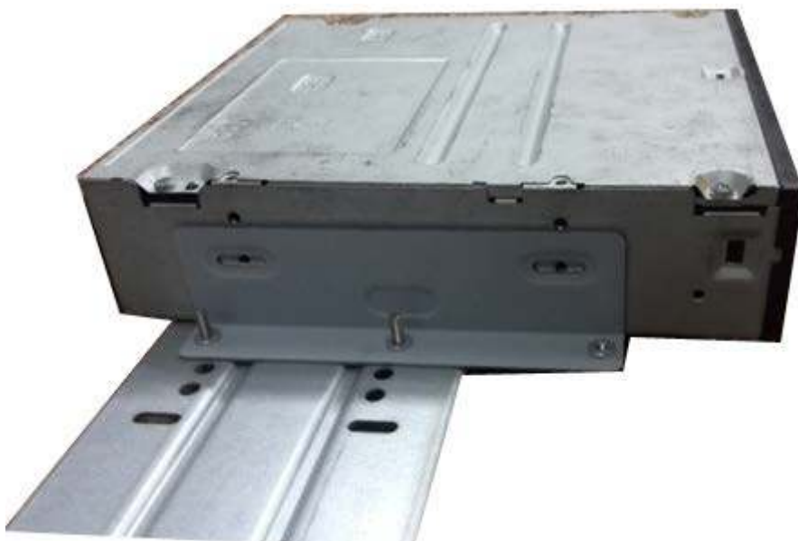
Figure 3-43 Install SATA burner
