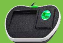
Multi-function scanner for card (IC & ID ) and fingerprint scanner
