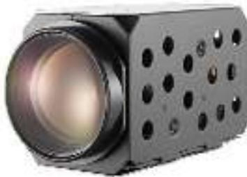
Hikvision iDS-2ZMN3207N(B) 2 MP 32 × Network Zoom Camera Module adopts 1/2.8" progressive scan CMOS chip. With the 32 × optical zoom lens, the camera module offers more details over expansive areas. This series of camera modules can be used for different types of PTZ cameras and positioning systems.
