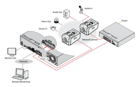
DirectIP™ NVR makes it easy to use cameras without extra network configurations.
