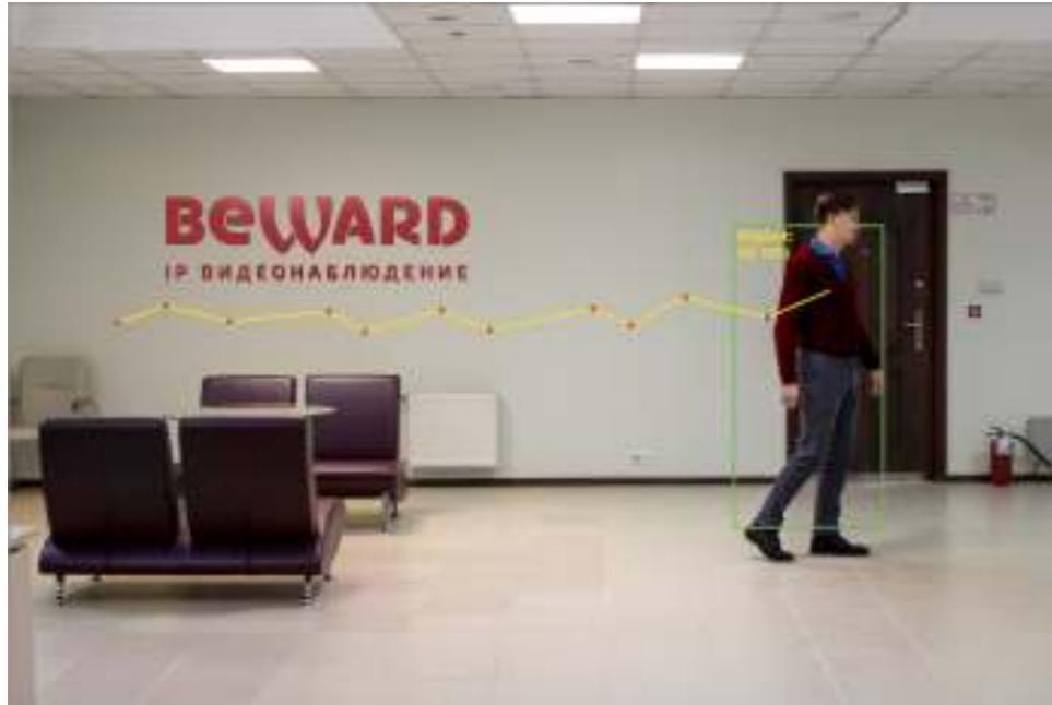
The interface includes configuration options for enabling person detection and tracking. A blue header bar at the top says "Детекция людей". Below it is a video feed showing a man walking across a room. A green rectangle highlights the man, and a yellow line traces his movement path.
