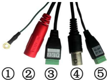
Figure 2-5 DS-2CZ2152P-IRA wiring definition
