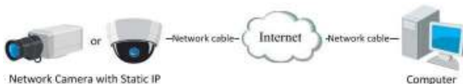
Figure 2-5 Accessing the Camera with Static IP Directly
