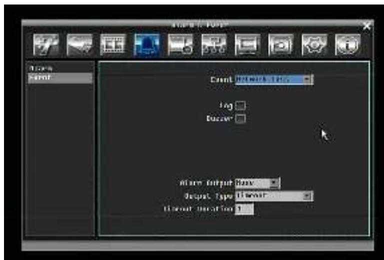
Figure 5-19 Alarm & Event Menu – Event – Network Loss
