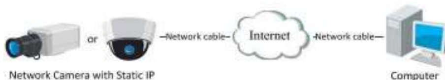
Figure 2-5 Accessing the Camera with Static IP Directly
