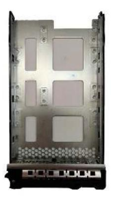
$\underline{\text{Step 3}}$  Put the disk into the disk tray and fasten the screws at the bottom of the tray. See Figure 2-3.
