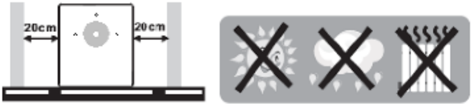
Figure 1. Placing of the UPS
