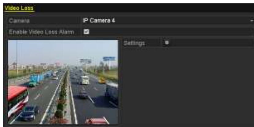
Figure 8.9 Video Loss Setup Interface
