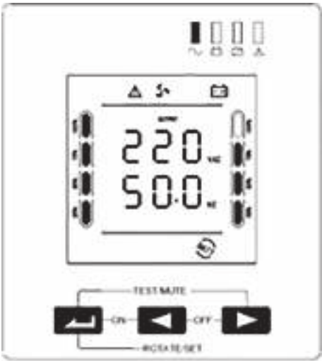
Figure 12. Display of the UPS
