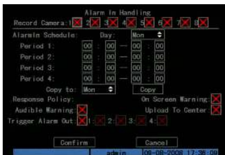
Fig. 5.24 Alarm in handling setup
