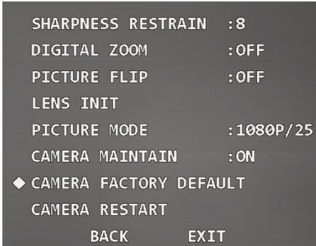
Figure 3-46 Restore the camera to factory default settings
