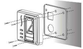
4) Use screws to fix the device and waterproof glue on the wall.
