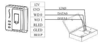
**Note:** 1) The recommended distance between device and access controller should not be more than 90 meters (If a longer distance or an environment with interference, please use the Wiegand signal extender).
