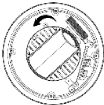
3. To detach PTZ camera from external housing, please turn it counterclockwise.
