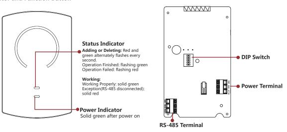
The power of wireless receiver is supplied by control panel on the model of DS-19A08-BN, DS-19A08-BNG, and DS-19A08-DNG. The power supply of the control panel is made by Channel Well Technology Co., Ltd., and meets LPS.
