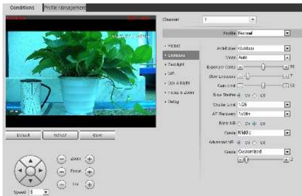
Figure 4-2 The exposure interface
