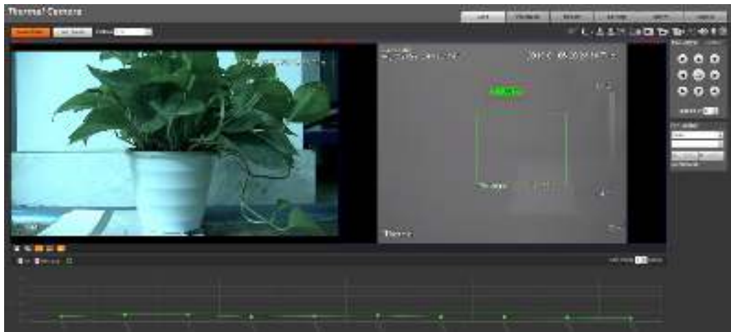
Figure 3-7 Real-time spot temperature measuring
