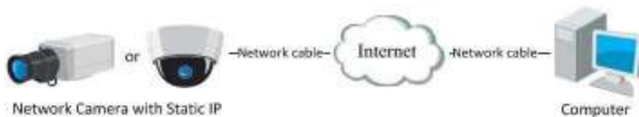
Figure 2-5 Accessing the Camera with Static IP Directly
