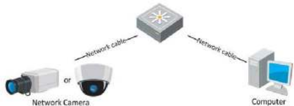
Figure 2-2 Connecting via a Switch or a Router
