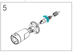
5 Push the waterproof cap body and cap into the RJ45 jack and rotate it.
